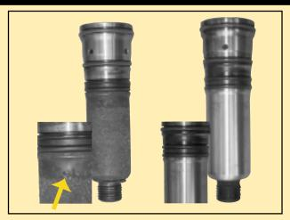
Injector sleeves from the same Bemco engine showed similar success for Cat ELC vs. conventional coolant. Note the deposits and severe pitting after 5,300 hours with conventional coolant (left) compared with the excellent condition of the injector sleeve with ELC after 10,013 hours of operation (right).
