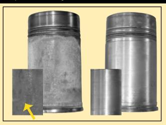
Bemco (the Caterpillar dealer in Botswana) compared engine component life using Cat ELC vs. conventional coolant. The liner on the left – from a Cat 3406 HEUI engine – operated 5,300 hours at the Gaborone Mine with conventional coolant. It had pitting, which penetrated the liner wall. The liner on the right from the same engine ran 10,013 hours with Cat ELC. The coolant side of the liner is like new.
