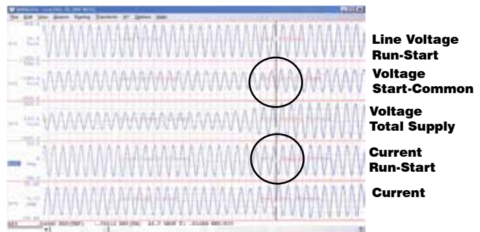
Figure 6. Start with Oversized Capacitor with out Safety Timing Circuit
